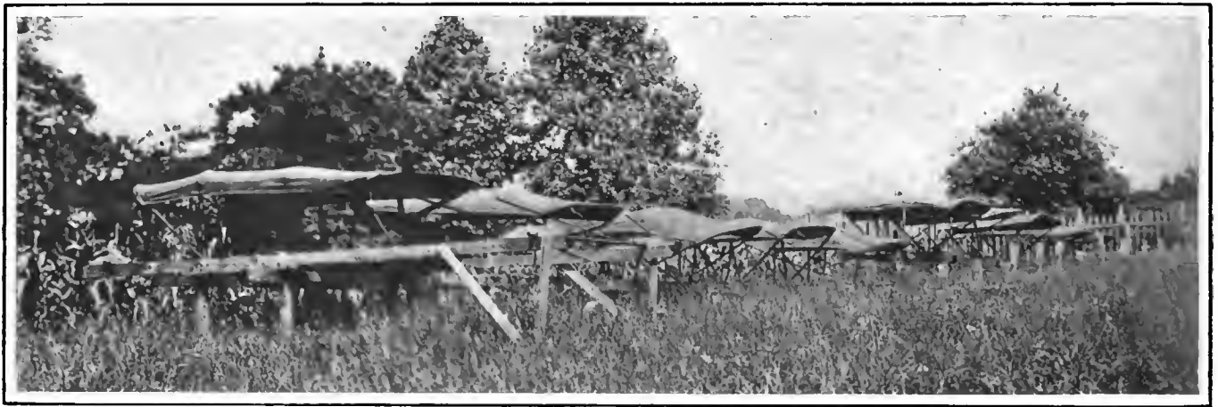
Tops of various manufacture tested by the Du Pont company for a year in an open field. They were opened and closed more frequently than if they had been mounted on cars in active service. Water was allowed to collect and stand on the tops for weeks and months at a time, as illustrated at the bottom of page 271
